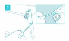
Remove the bottom hinge by removing the screws. Swap the adjustable foot from left side to right side removing the fixed screw in the left side first.
