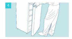
Remove the lower door from the bottom hinge pin. Tilt the fridge backwards and rest it on a firm surface.
