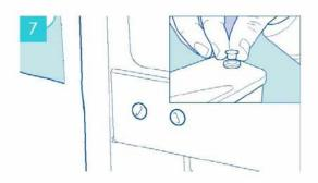
Reverse the blanking plugs. Remove the door hinge cap in the top of the freezer door and insert it on the opposite side of the door.
