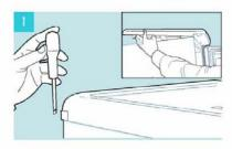
Undo the four retaining screws on the rear of the worktop and remove the worktop
