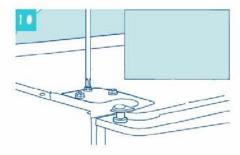
Refit the top hinge while refitting the upper door. Do not fully tighten screws.
