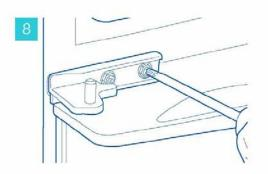
Replace the central hinge while refitting the lower door, To assist with final adjustment do not fully tighten the hinge screws.
