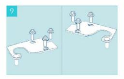
Unscrew the hinge pin from the top hinge using the spanner. Turn the hinge over and replace it in the same slot. (Reversed)
