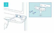
While supporting the lower door, remove the central hinge by removing the 2 screws.
