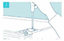
Undo the retaining screws of the top hinge and remove the top hinge. Then remove the upper door and put it in a safe place.
